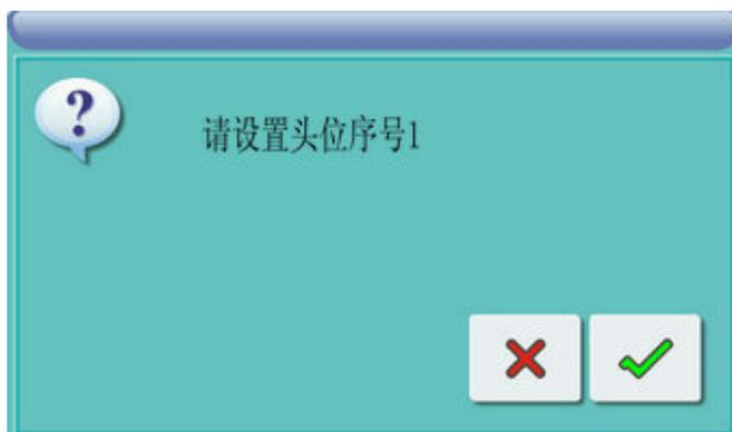
System ask you to set head serial number “1”, then dial three position switch on this head to down position. After that, dial the switch to middle position. If success, system will increase head serial number to “2”. Other heads are the same.
