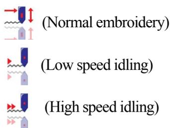
After set low speed idling
