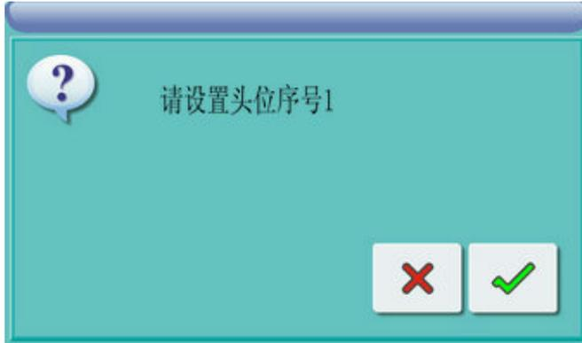
System ask you to set head serial number “1”, then dial three position switch on this head to down position. After that, dial the switch to middle position.
